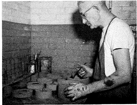
BILL SHEA assembles the four parts of a dry sand mold for a Wheelabrator impeller casting which will be poured of steel. The various parts of the mold are held together with core paste.
