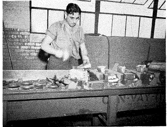
ARTHUR CROOK uses a hammer to remove baked-on sand from an electric heater casting. Later the surplus metal is sawed off and the casting is Wheelabrated to remove the baked-on sand.
